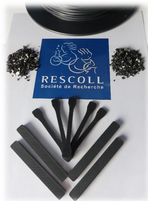
HIPS recycled filament & printed coupons
