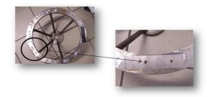
Fig.5. Debonding with adhesive failure of SiC pieces bonded on Invar crown
