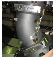
Fig.6. Proof test of structural Gaia torus Part.
