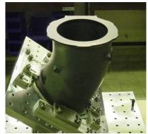
Fig.7. Structural Gaia torus Part after debonding
