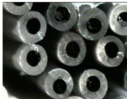
Image of bi-component fibers incorporating non-encapsulated PCMs
