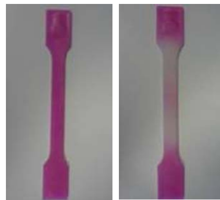
Thermochromic EVA plates (color change at 63°C)
