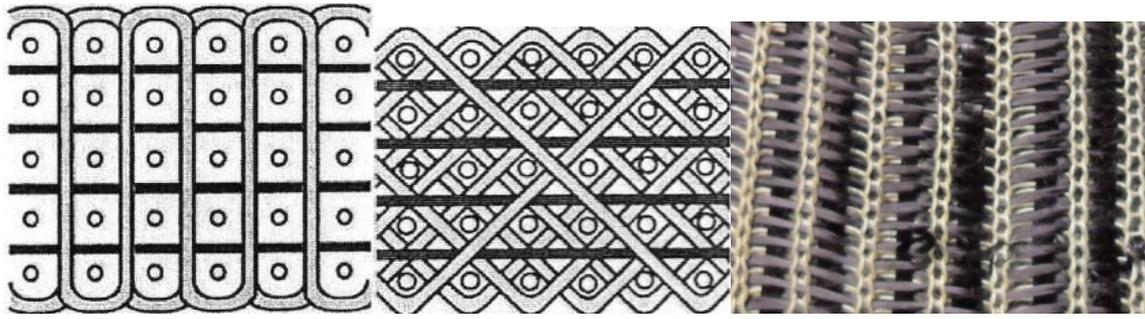
**Figure 7.** A 3D orthogonal Interlock, an Angled Interlock and a 3D textile developed by JTT Composite.
