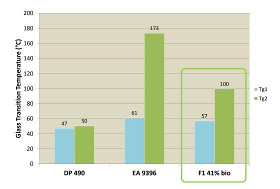
• Glass transition temperature value of bio based formulation is between that of commercial adhesives
