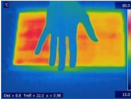
CTAG will develop a heating seat. The resulting prototype will reach a thermal leap of 15°C with consumption lower than the conventional electric resistances. **It will work with a 12V voltage**, similar to a car battery. This is considered to be a secure working voltage so it could be used in humid
