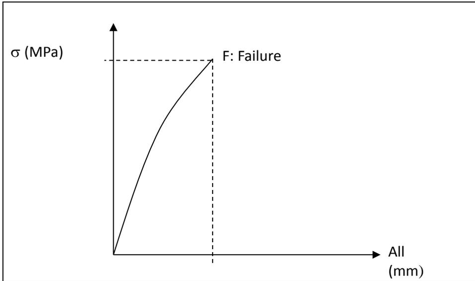
$\sigma_F$  : Tensile lap shear strength =  $F/S_0$
