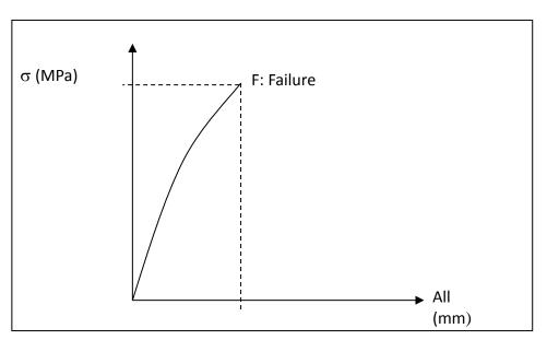
$\sigma_{\rm F}$ : Tensile lap shear strength = F/S<sub>0</sub>
