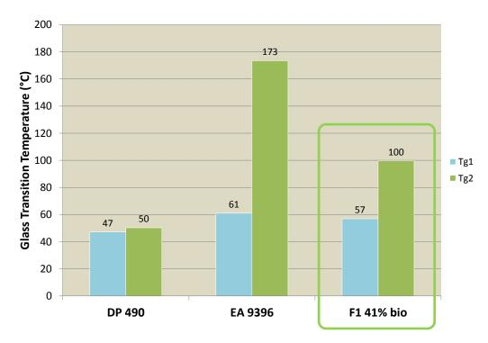
Glass transition temperature value of bio based formulation is between that of commercial adhesives
