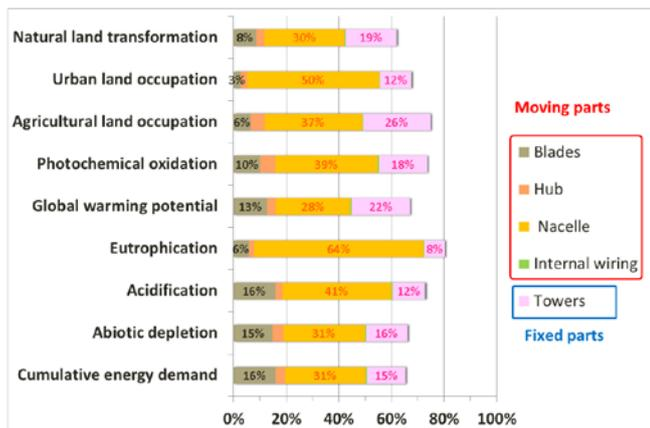
Figure 4: Contribution of manufacture of mobile and fixed components to impact of the wind plant.
