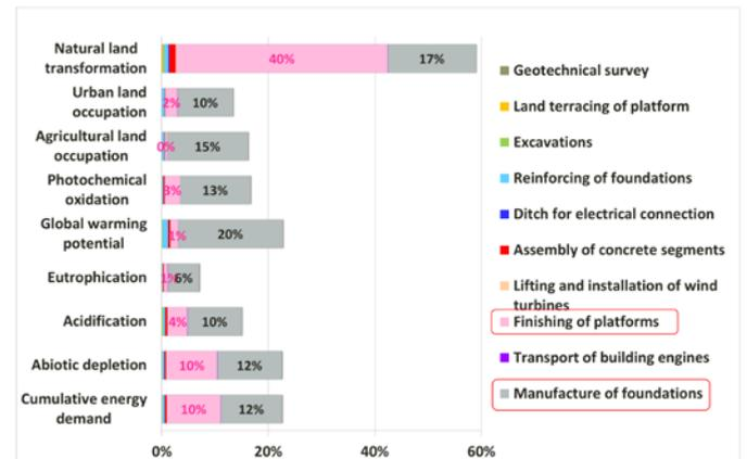
Figure 5: Contribution of the construction stage to impact categories.
