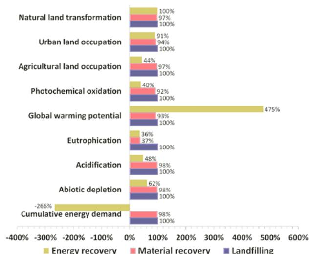
Figure 6: A comparison of the effects of considering different scenarios of blade end of life.
