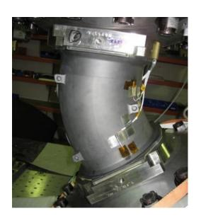
Thermal activation of the bonded system
