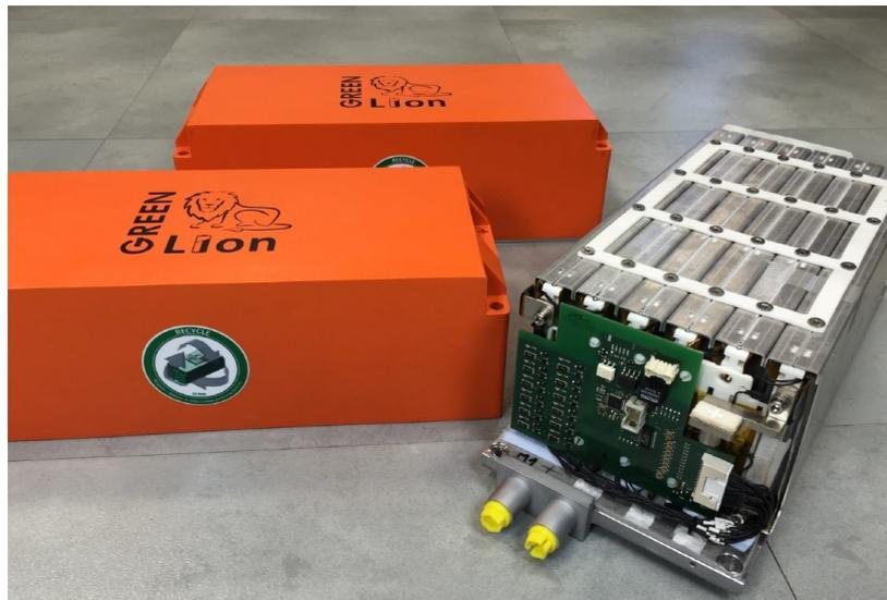
**Figure 1: Module Li-Ion GREENLION**
