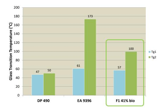
Glass transition temperature value of bio based formulation is between that of commercial resins
