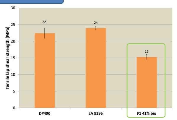
• Bonding properties of biobased formulation should be improved
