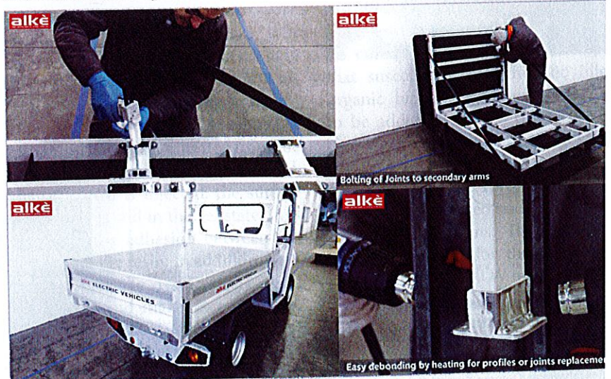
Fig.7: Assembly of the full cargo bed by adhesive join and easy debonding picture
