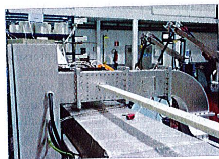
Fig. 1: Antenna MW design for the curing of the AL.KÉ's profile (automotive sector)
