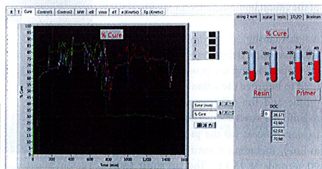
Fig.5: Online prediction of the degree of cure from the 4 cure sensors. At the top right-hand-side the real-time degree of cure are displayed for the 2 sensors in the resin region and the other 2 cure sensors at the primer area
