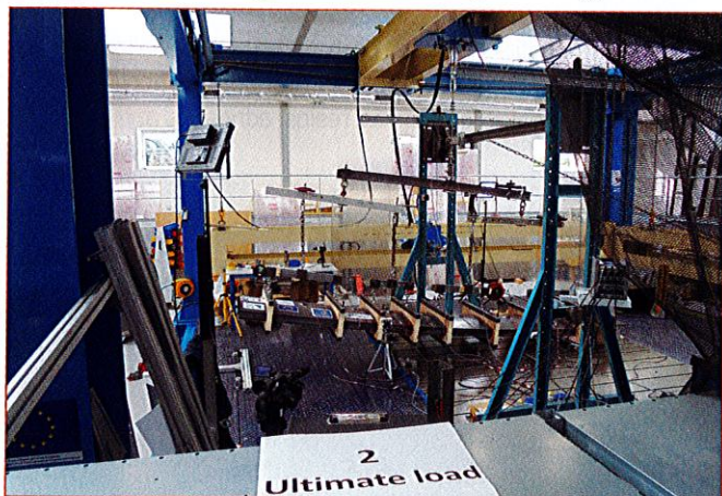
Neofac wing tested up to 13G on Rescoll's benches
