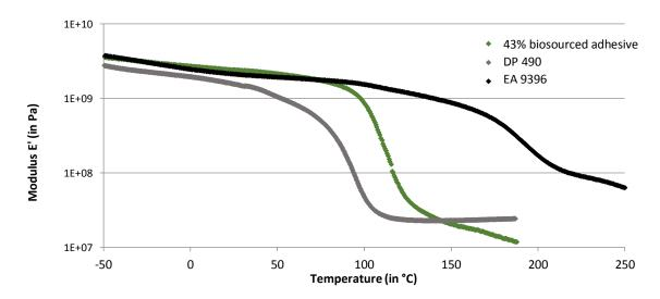
Glass transition temperature of biosourced adhesive is around 100°C. Common epoxy adhesive as DP490 display lower thermal properties than our biosourced adhesive.
