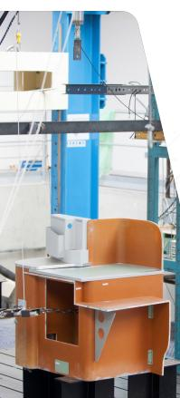
Static and fatigue tests on specimen: · Sandwich panels
