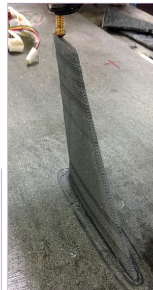
Vertical stabilizer during printing with ABS/Carbon fibre
